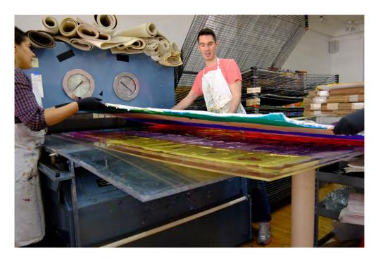
the paper laid face down on top. The button is pushed and the press exerts 750 tons of downward pressure forcing the paper into the letters. With the interaction of so many uncontrollable variables (temperature, humidity, viscosity and atmospheric pressure) there is no predicting what the paint will do.
